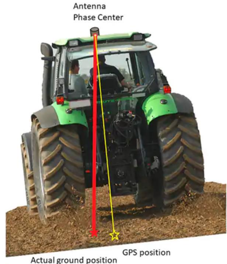
Figure 2: GPS cannot determine orientation, so slopes could result in errors when determining the equipment's actual ground position. (Image source: Richard A Quinnell)
