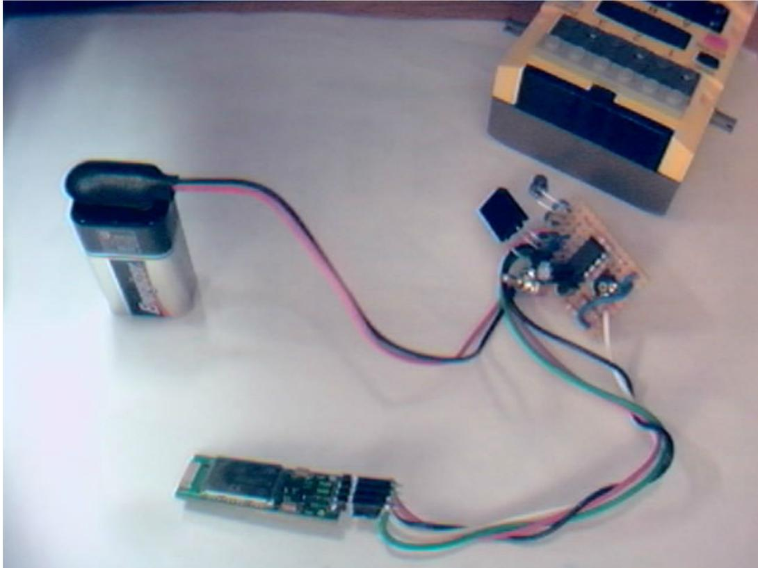
Figure 5. The device is powered from 9V battery. The BlueSmiRF module can be unplugged and used in other designs when needed. It can also be placed comfortably at a separate location - such as on top of the robot for best RF transmission.
