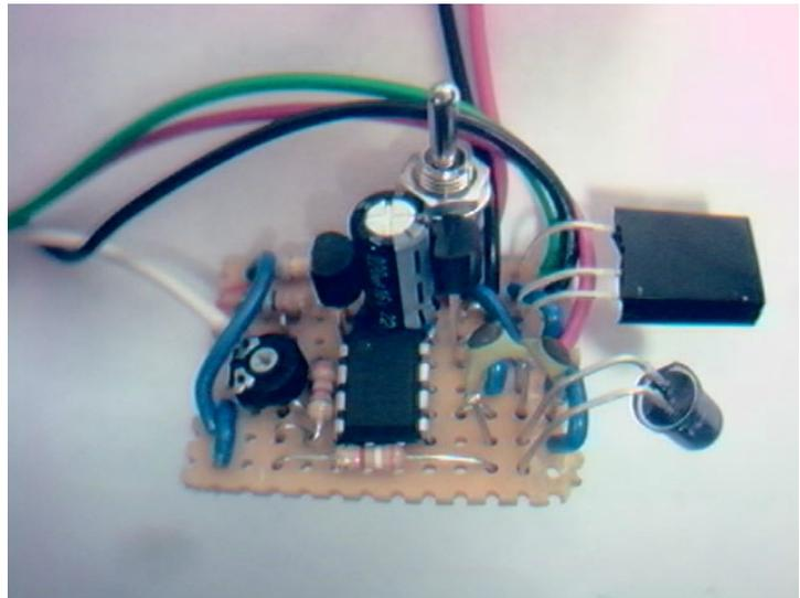
Figure 4. Serial to IR bi-directional converter. The board on the left is from the point of view of the parts. The switch is installed between the two pads, where the 9V battery cable connects. This design utilizes two parallel 47pF capacitors instead of the single 100pF shown on the schematic above.
